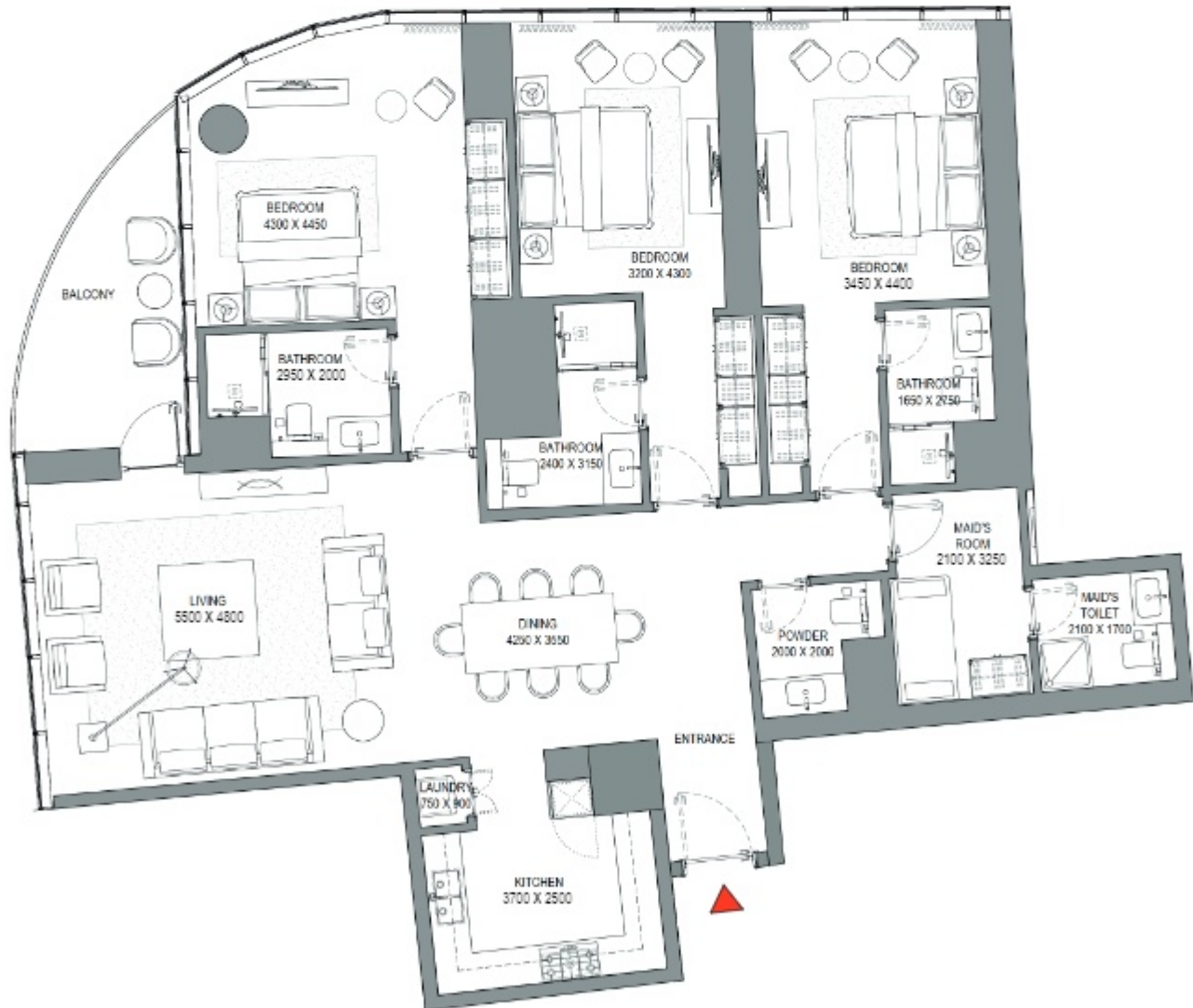
TYPICAL FLOOR PLAN LEVEL 12-23
